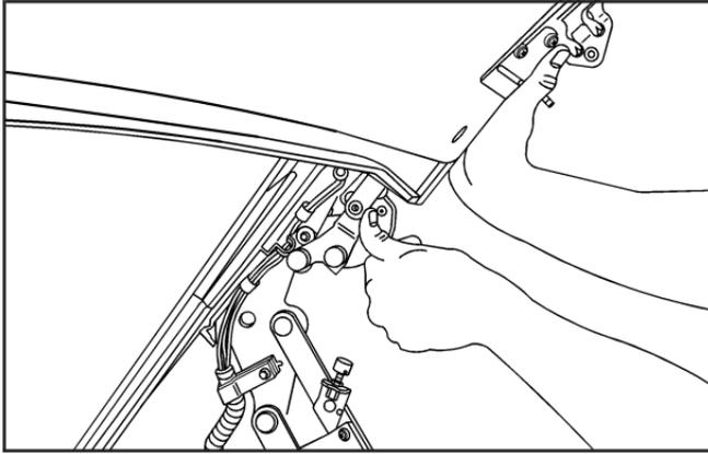
7. Push both sides of the rear tonneau over-center link up until they stop to lock the linkage.
