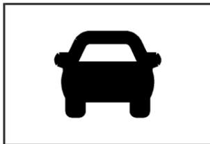
The vehicle ahead symbol only appears on the HUD when a vehicle ahead is detected in your path.
