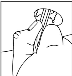
18. While holding the rear of the top down, insert the wrench into the bolt in the plug opening in the headliner. Turn the wrench counterclockwise until it stops to fully open the latch jaws around the pins.
