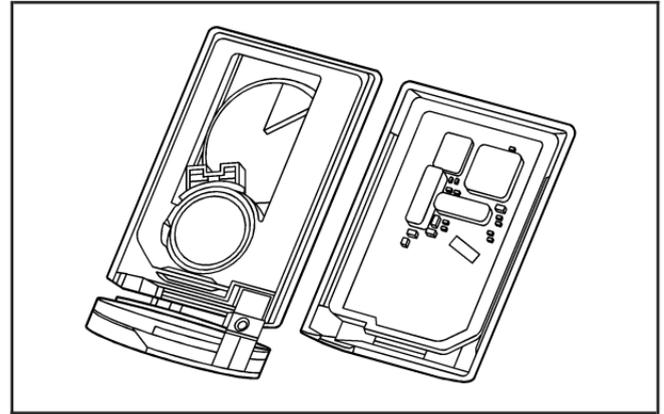
1. Insert a flat object with a thin edge into the slot on the side of the transmitter and separate the bottom half from the top half.
