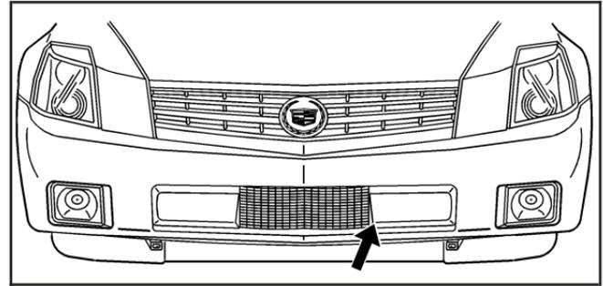
Clean the surface with a 50/50 mixture of isopropyl alcohol and water on a dampened cloth. After cleaning the fascia lens, try to engage Adaptive Cruise Control. If this does not fix the problem, you may have to remove the fascia lens and clean the inside of the fascia lens and radar lens.
