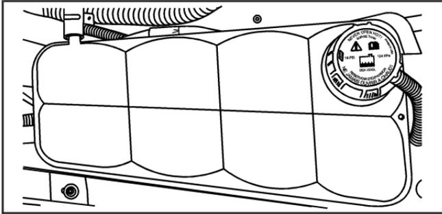
The engine coolant surge tank is located toward the rear of the engine compartment on the driver's side of the vehicle. For more information on location, see *Engine Compartment Overview on page 6-12*.
