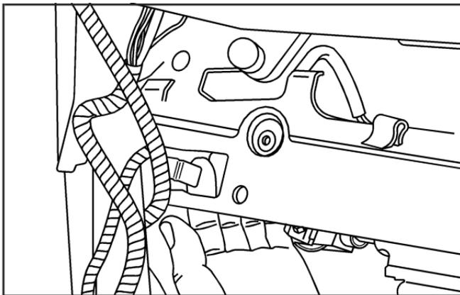
10. Reach behind the square hole and push the front tonneau over-center link up. The front tonneau should pull up easily. If it does not, push the over-center link up more.
