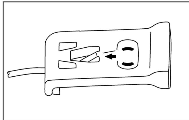
If you are outside the vehicle, there is a door release tab in the trunk. The tab is located behind a panel on the driver's side of the trunk. Pull the handle to unlock and unlatch the driver's door. See *Trunk* on page 2-13 for information on opening the trunk during a loss of power.
