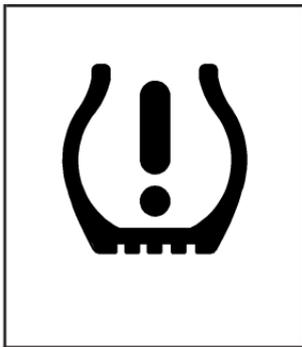
When a low tire pressure condition is detected, the TPMS illuminates the low tire pressure warning light, located in the instrument panel cluster.
