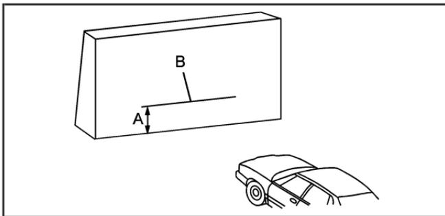
4. At the wall or other flat surface, measure from the ground upward (A) to the recorded distance from Step 3 and mark it.
