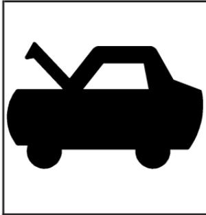
1. Pull the lever with this symbol on it. It is located on the lower left side of the instrument panel.
