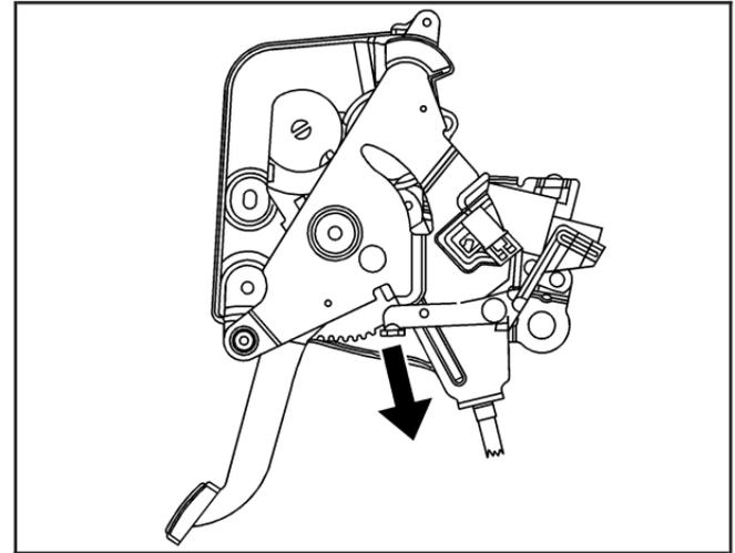
Reach under the driver's side of the instrument panel and pull down on the manual release lever, which is located behind the parking brake pedal. Pull down on the yellow tab. If the parking brake does not release, you should have your vehicle towed to your dealer for service.
