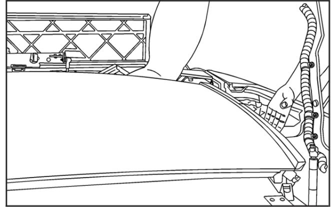
14. Hold the top in the front and side and lift the top out of the stored position.
