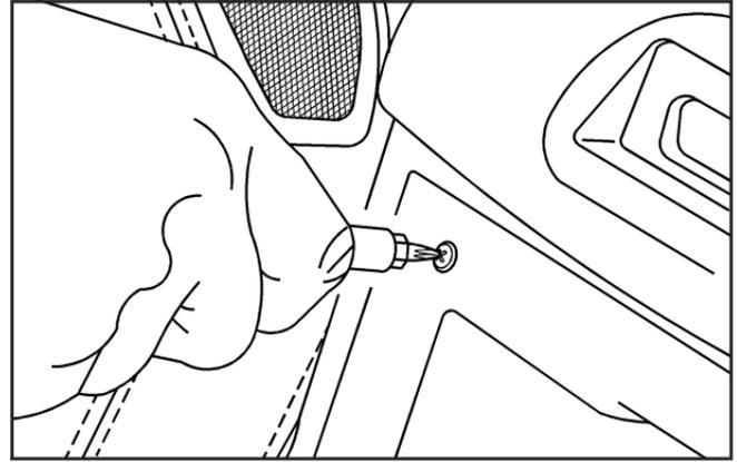
9. Remove the upright center storage compartment. Use the wrench to remove the four screws holding the storage area in place.
