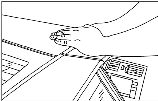
20. From outside the vehicle, push down on both rear corners of the top to make sure it is completely locked into place.
