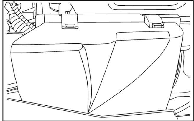
2. Move the clasps on the top of the engine air cleaner/filter cover forward to unlatch the cover.
