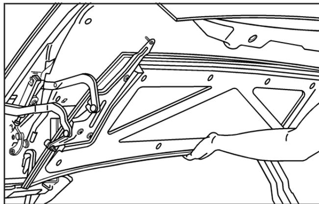
6. Move the rear tonneau rearward and up to the stored position. Pull from the center of the tonneau to keep pressure even. The rubber bumper on each corner will fit against the underside of the trunk decklid.
