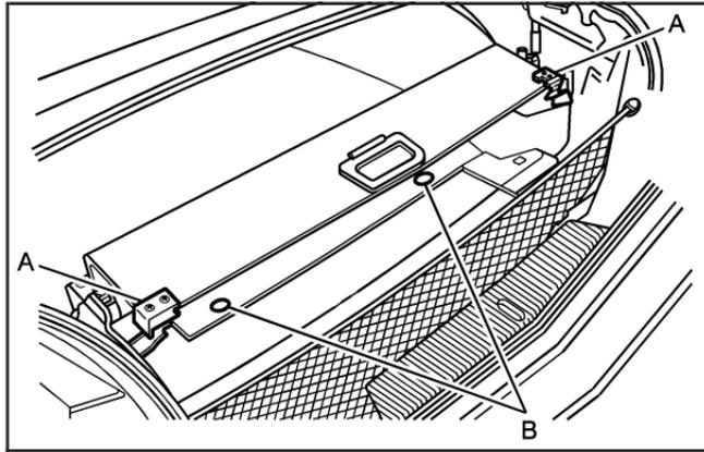
There is a cargo divider located in the trunk to keep cargo from getting in the way of the retractable hardtop. The cargo divider must be in place for the top to move.
