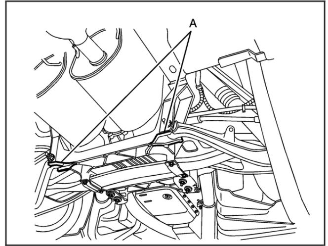
1. Locate the rear lifting points (A), according to the illustration shown.
