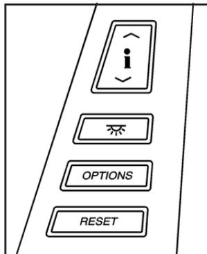
The Driver Information Center (DIC) buttons are located to the right of the steering wheel on the instrument panel, near the air outlets.
