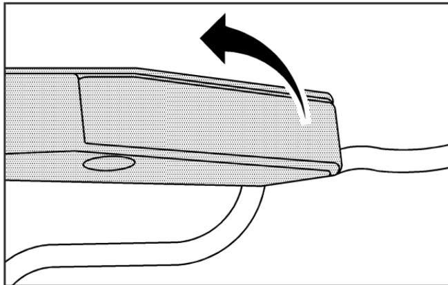
If you are inside the vehicle, use the door release handle located on the floor next to each seat. Pull the handle up to unlock and unlatch the door.
