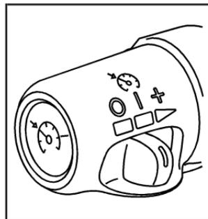
The cruise controls are located on the end of the multifunction lever.
