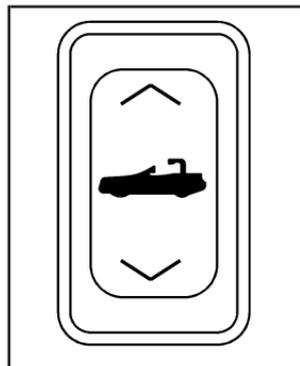
5. Push and hold the top of the retractable hardtop button located behind the shift lever. The windows will automatically lower and the top will raise. A chime will sound when the top has raised completely.
