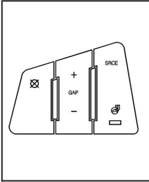
Use the GAP button on the steering wheel to adjust the follow distance between your vehicle and other vehicle's.
