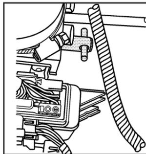
4. Find the hydraulic pump under the carpet on the rear driver's side of the trunk. Open the valve by turning it counterclockwise with your hand until it stops.
