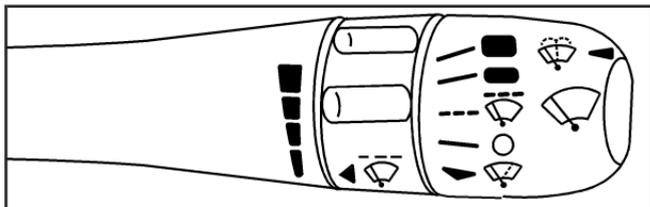
Use the lever located on the right side of the steering column to operate the windshield wipers.
