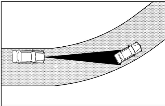
Adaptive Cruise Control might detect a vehicle that is not in your lane and apply the brakes.
