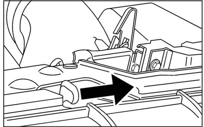
2. Then go to the front of the vehicle and find the secondary hood release lever. The lever is located under the hood near the center of the vehicle. Move the release lever to the right and raise the hood.
