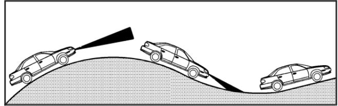
How well Adaptive Cruise Control works on hills depends on your speed, vehicle load, traffic conditions, and the steepness of the hills. It might not detect a vehicle in your lane while driving on hills. While going up steep hills, you might want to use the accelerator pedal to maintain your vehicle speed. While going downhill, you might have to brake to keep your vehicle speed down. Applying the brake disengages the system. You may choose not to use Adaptive Cruise Control on steep hills.
