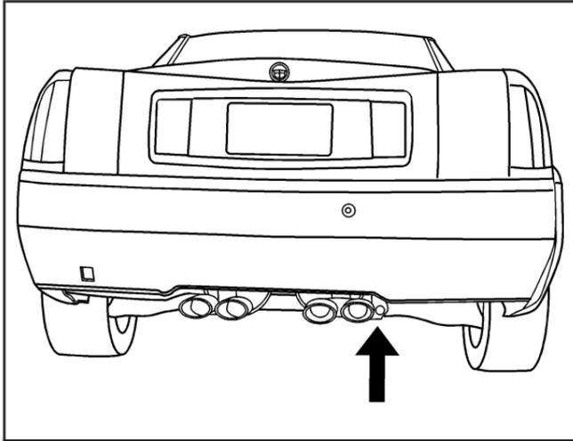
The rear lifting points can be accessed from the rear of the vehicle, on either the driver's or passenger's side.
