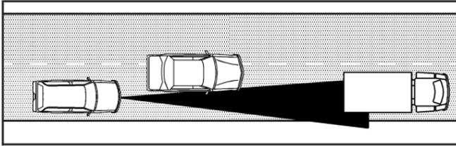
If another vehicle enters the same lane as you, Adaptive Cruise Control will not detect the vehicle until it is completely in the lane. Be ready to take action and apply the brakes yourself.
