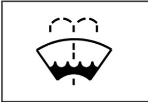
Open the cap with the washer symbol on it. Add washer fluid until the tank is full. See *Engine Compartment Overview* on page 6-12 for reservoir location.
