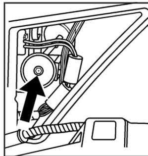
8. Turn the vertical aiming screw until the headlamp beam is aimed to the horizontal tape line.
