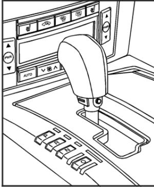
To use this feature, move the shift lever from the DRIVE (D) position to the left and into the driver shift control gate.
