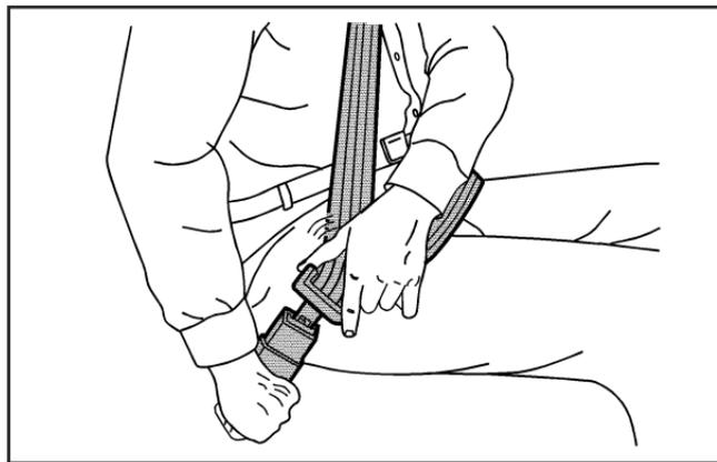
3. Push the latch plate into the buckle until it clicks. Pull up on the latch plate to make sure it is secure. If the belt is not long enough, see *Safety Belt Extender on page 1-23*.
