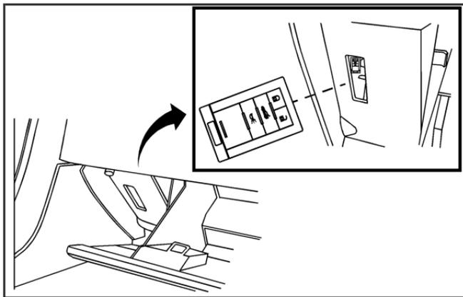
2. Place the new, unrecognized transmitter in the glove box transmitter pocket with the buttons facing to the right.
