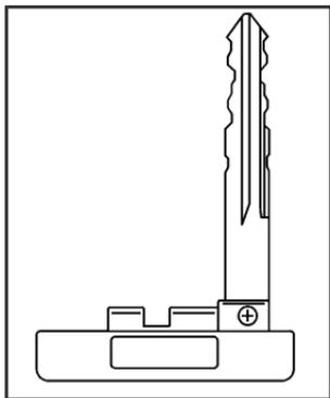
This key, located inside the keyless access transmitter, can be used for the glove box and the trunk, if vehicle power is lost. See *Trunk on page 2-13* for more information.
