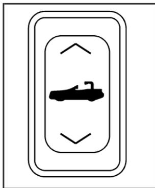
5. Push and hold the bottom of the retractable hardtop button located on the console behind the shifter lever.
