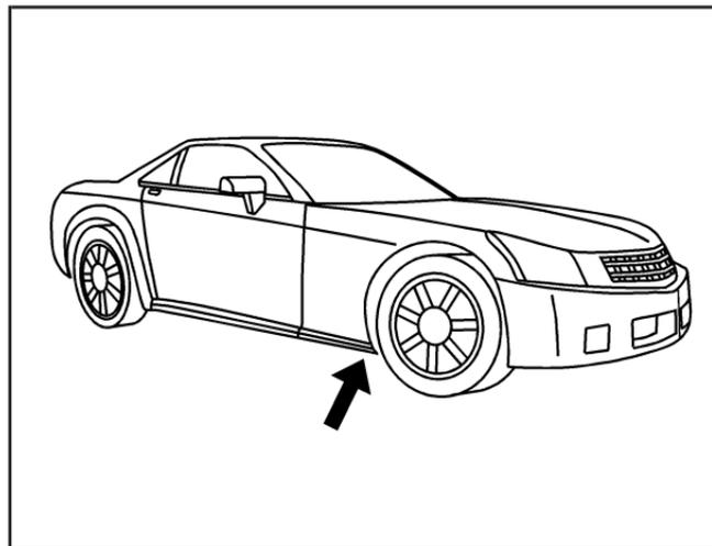
The front lifting points can be accessed from either side of your vehicle, behind the front tires.
