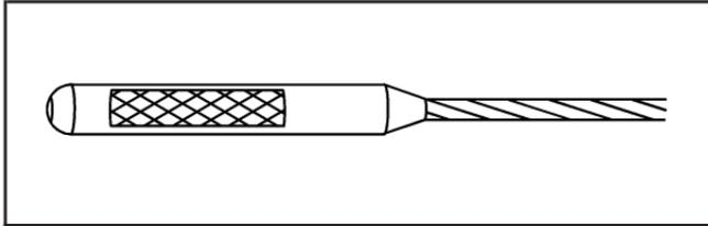
If the oil is below the cross-hatched area at the tip of the dipstick, add at least one quart/liter of the recommended oil. This section explains what kind of oil to use. For engine oil crankcase capacity, see *Capacities and Specifications on page 6-97*.
