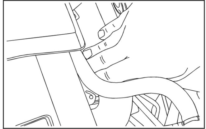
3. Fill the coolant surge tank with the proper mixture until the level inside the surge tank stabilizes at the FULL COLD mark on the front of the surge tank.
