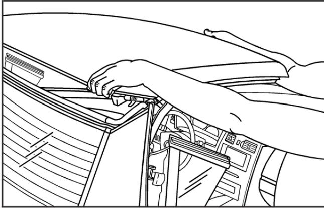
15. Hold the top in the front and the rear and lift the top until it is almost closed. Be careful not to pinch your fingers between the rear of the top and the rear window.
