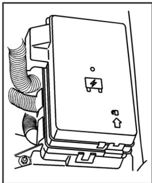
The underhood fuse block is located next to the engine on the passenger's side of the vehicle.
