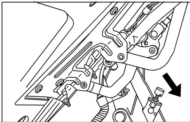
5. Pull both sides of the rear tonneau over-center link down to unlock the linkage.
