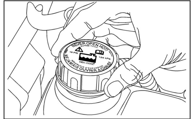
1. You can remove the coolant surge tank pressure cap when the cooling system, including the coolant surge tank pressure cap and upper radiator hose, is no longer hot. Turn the pressure cap slowly counterclockwise.
