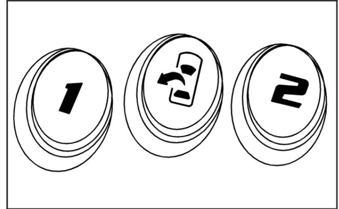
Your vehicle is equipped with the memory package. The controls for these features are located on the driver's seat, and are used to program and recall memory settings for the driver's seating positions.
