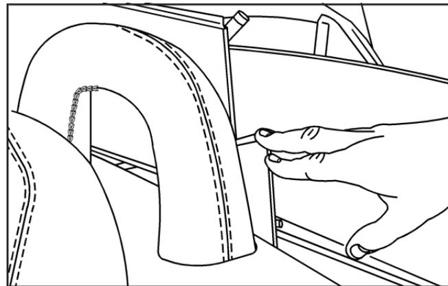
11. Manually move the front tonneau to the open position. Once the front tonneau is open, fold the side wings by gently pressing them in. Do not force the wings. If they are hard to move, make sure the front tonneau is open all the way.
