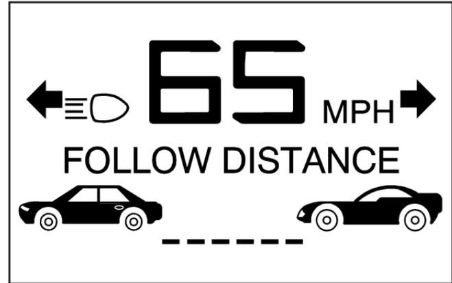
A graphic on the HUD indicates the selected following distance. This picture shows a maximum follow distance. The vehicles will move closer together as you select a smaller following distance.
