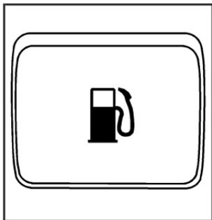
The fuel door release button is located on the left side of the instrument panel. The button only works when the vehicle is in PARK (P) or NEUTRAL (N) and the valet lockout button is in OFF.
