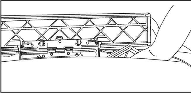
12. Reach in from the side of the vehicle and under the top to remove the headliner plug. The plug will be located in the center of the top near the front.
