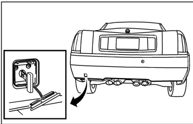
The key cylinder is located behind a cover on the lower rear fascia on the driver's side of the vehicle. Open the door to access the key cylinder.
