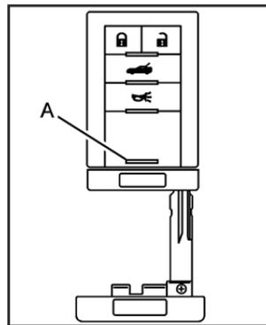
To remove the key, press the button (A) near the bottom of the keyless access transmitter, and pull the key out. Never pull the key out without pressing the button.
