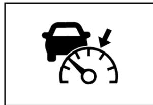
This symbol appears on the Head-Up Display (HUD) to indicate that Adaptive Cruise Control is active.
