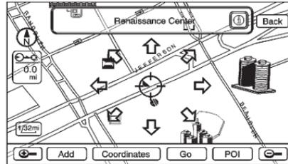
While scrolling the map, traffic condition icons may appear. To receive information about the traffic condition, place the cross hairs over the traffic condition icon. After selecting the **i** (information) screen button, the type of traffic condition, the street name, and a description of the traffic condition appears on the display. See “Scrolling the Map” under *Maps on page 36* for more information.
