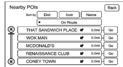
**Nearby POIs:** Press to display the list of available POIs for the selected POI categories. The list provides the POI icon, the name, the direction, and the distance to the POI from the vehicle's current position. Use the scroll arrows to move up and down the list. Use the Sort by Dist (distance), Icon, Name, and, on Route as desired.
