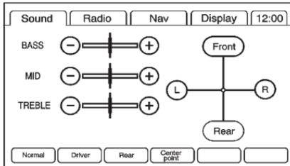
Press the CONFIG control button to adjust several of the system's features and preferences. The last selected menu screen is the screen that displays; Sound, Radio, Nav (navigation), Display, or clock.
