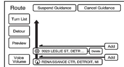
**Add:** Press this screen button from the Route screen. This feature allows up to three waypoints to be added to the current route, between one start point and final destination. Once a waypoint has been added, the points can be edited or deleted.
