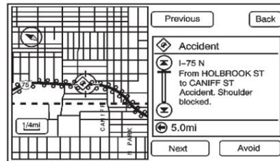
2. Select a traffic condition to view it on the map. The map screen displays with the area of the traffic condition shown. Press the Next or Previous screen buttons to view the accident locations that are on the list.
