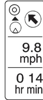
The distance and time to destination symbol indicates the distance and the estimated time remaining to the final destination or arrival time, depending on the option selected.
