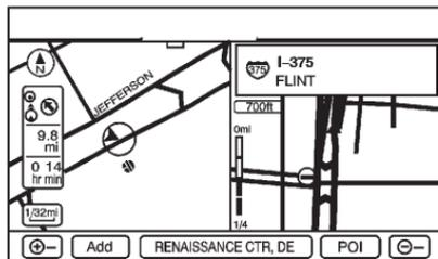
When approximately 0.4 km (1/4 mi) from the next maneuver, the screen displays the name and a detailed view of the next maneuver.
