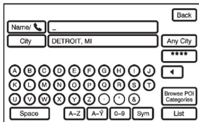
**Point of Interest:** The Point of Interest (POI) destination entry method allows selection of a destination by providing the system with a POI name, a city name, or selecting the POI from the POI list.
