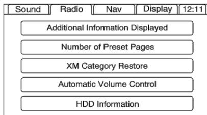
Press CONFIG to enter the menu screen, then press CONFIG repeatedly until Radio is selected or press the Radio screen button to make radio system changes.
