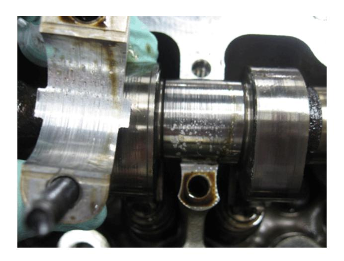
1. Inspect for damage to the cam caps journals and camshaft journals on the heads (obvious signs of metal through the cap).
