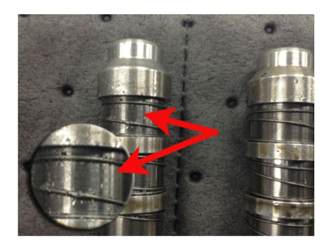
1. Inspect the oil control solenoids for metal debris. This shows the oil filter is in by-pass and unfiltered oil with bearing debris was pumped into the oil lubrication galleys, throughout the engine.
