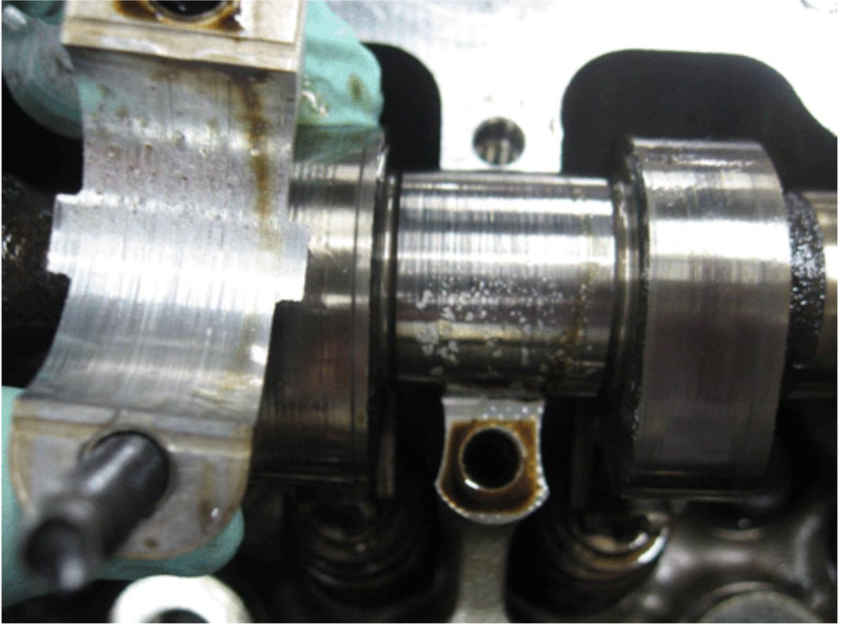
1. Inspect for damage to the cam caps journals and camshaft journals on the heads (obvious signs of metal through the cap).
