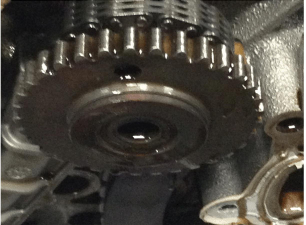
1. Inspect the timing chain idler sprockets for stiffness when turning (Should turn smooth and free).
