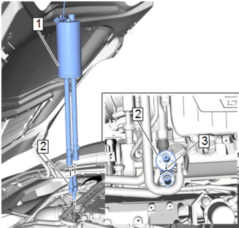
1. Insert the other end of the *GE-52079-10* adapter (2) into the fill port tee.
