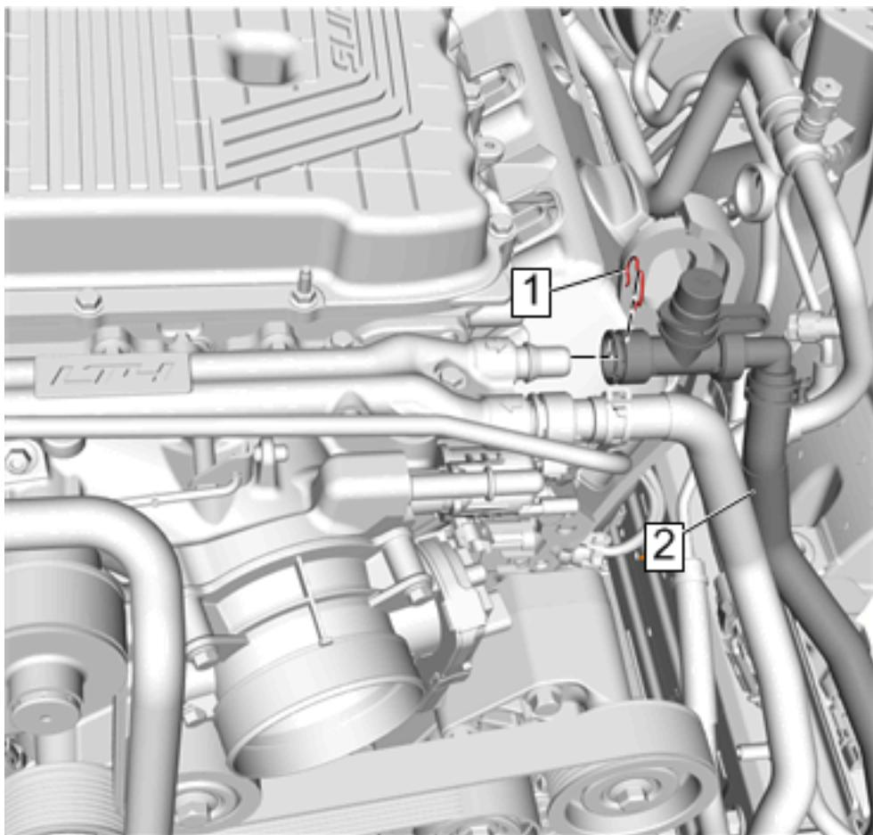
1. Remove the charge air cooler coolant hose retainer (1).
