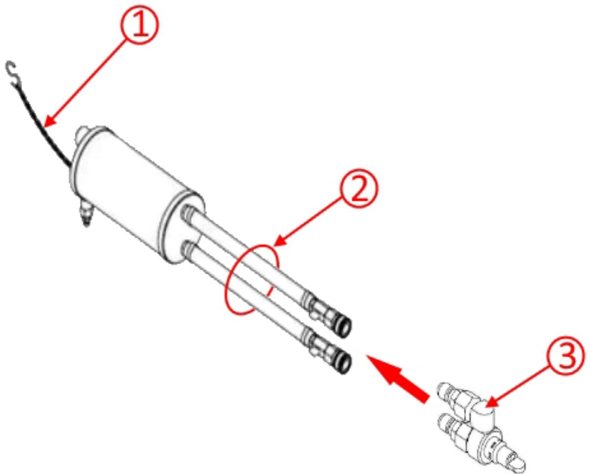
1. Attach *GE-52079 Tool, Coolant System Fill* lines (2) to *GE-52079-10 Adapter, Coolant System Fill Tool* (3).
