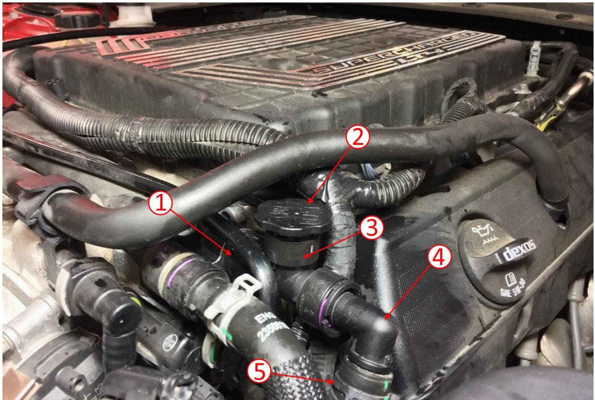
1. Assemble the new fill port (3) with cap (2) and 90 degree elbow (4).
