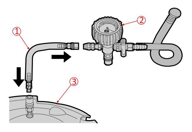
1. Attach the vacuum hose (1) to the vacuum gauge assembly (2) and the vacuum tank (3).
