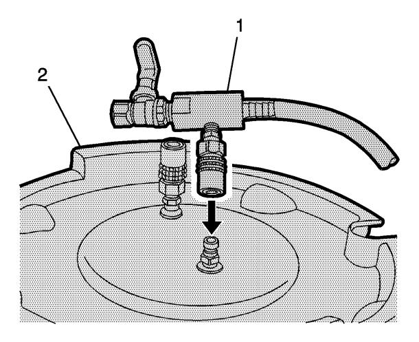
1. Attach the venturi assembly (1) to the vacuum tank (2).
