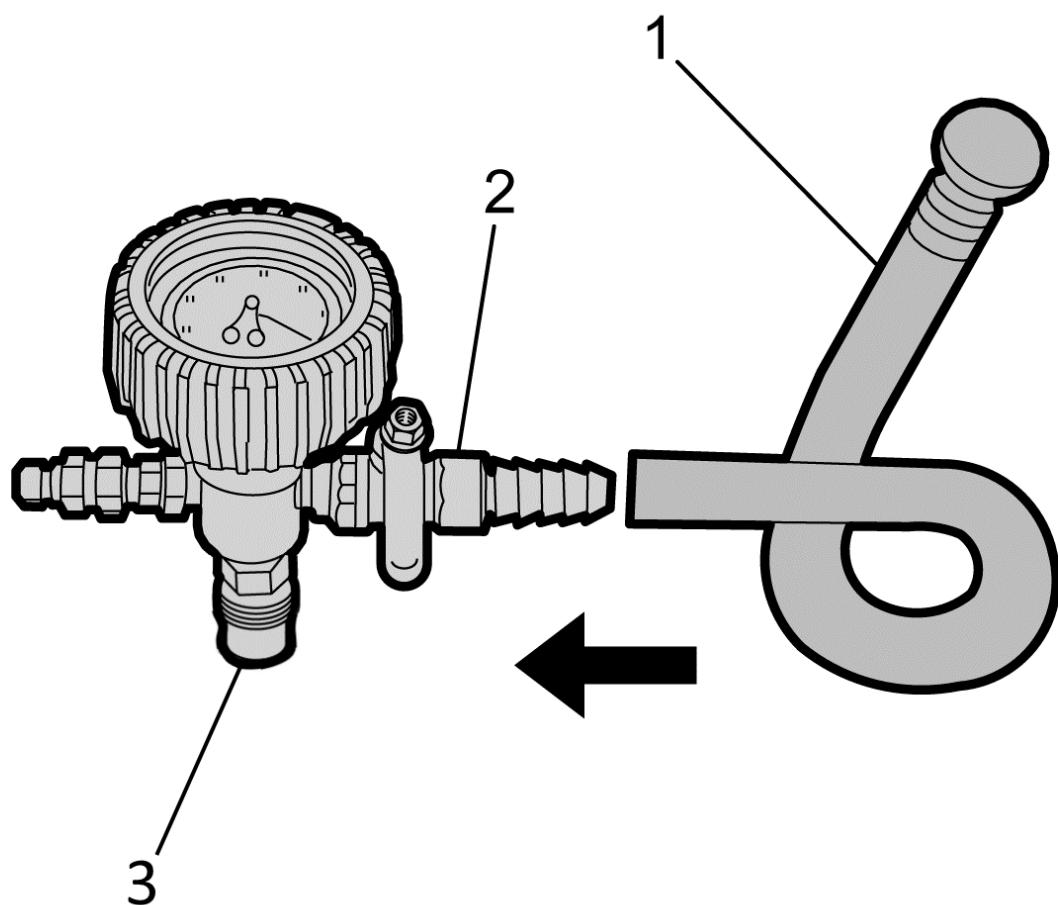
1. Attach the vacuum gauge lower port (3) to top port of the *GE-52079* tank.
