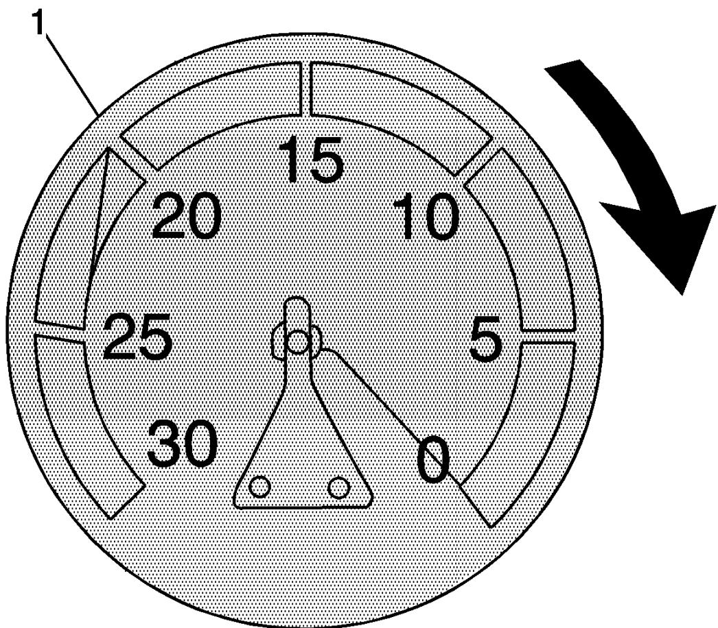
1. Once the vacuum gauge (1) reaches zero, close the valve on the vacuum gauge assembly and repeat steps 10-16 at least two more times.
