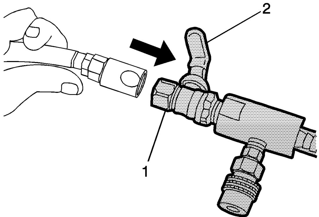
1. Attach a shop air hose to the venturi assembly (1).
