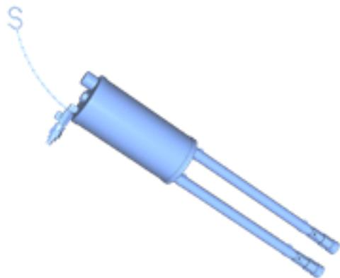
1. Add .5 qt (.5 L) of coolant to the system through service tool GE-52079.
