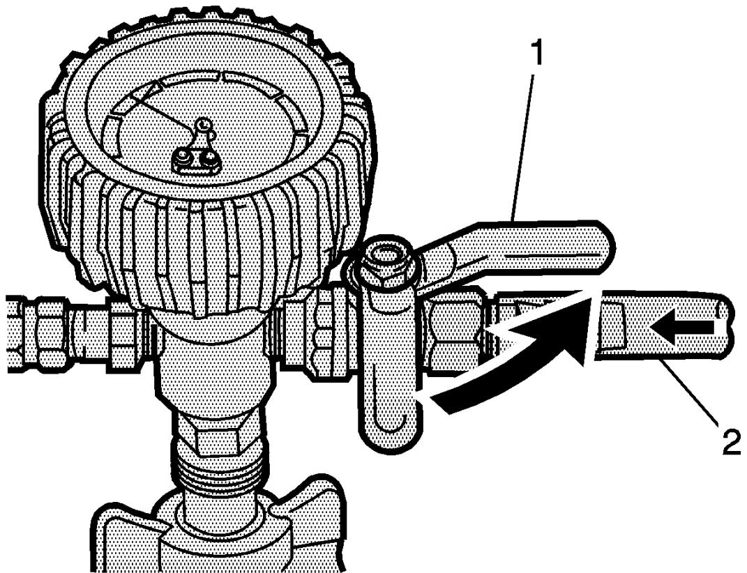
1. Slowly open the valve (1) on the vacuum gauge assembly (2).
