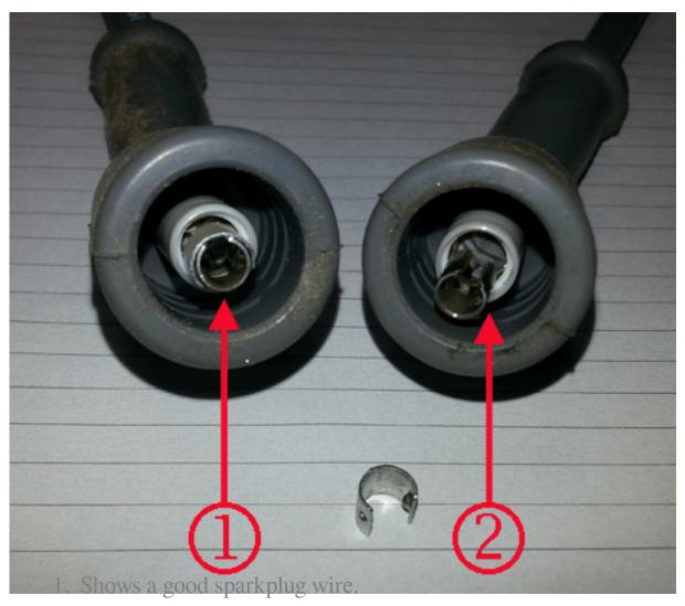
2. Shows the wire with the C clip missing.
