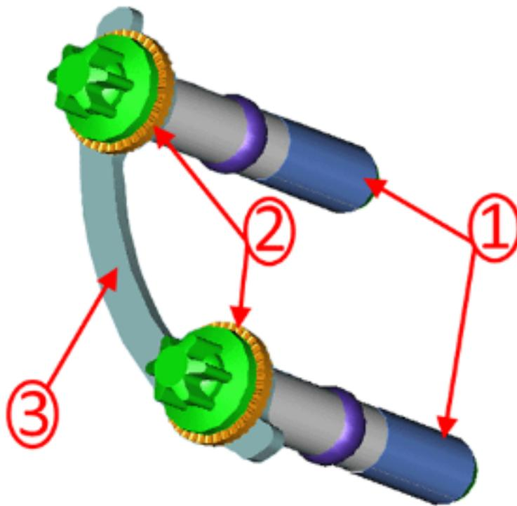
This bulletin advises the Service Technician of new retainer assemblies that are required to be installed during any repair that requires the half shaft bolts to be removed or replaced.
