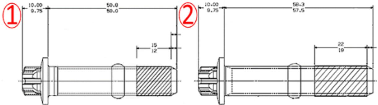
Service stock half shafts may include POA retainer assemblies that have the shorter bolt (1), these assemblies may require to be exchanged with new retainer assemblies that have the longer bolts (2).
