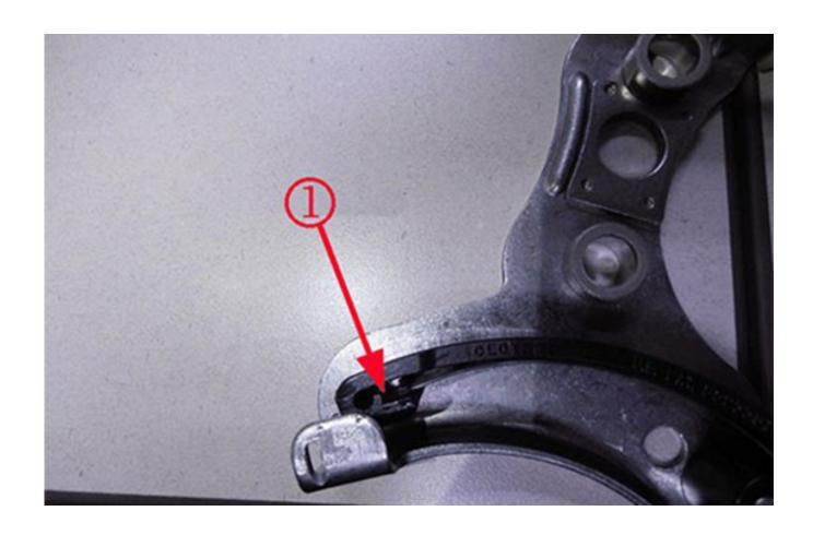
In addition, a broken tensioner shoe (Fig. 20) may allow the spring to rub a hole in the oil pump.
