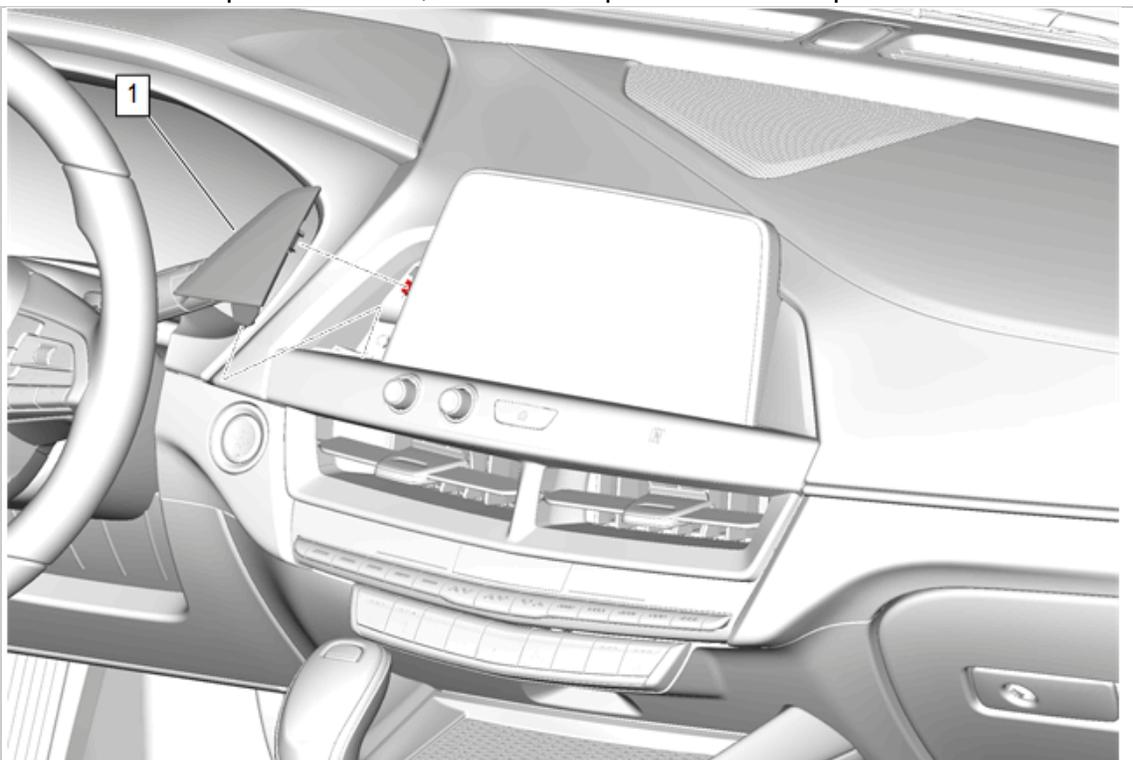
2. Instrument Panel Radio Front Trim Plate (1) » Remove
