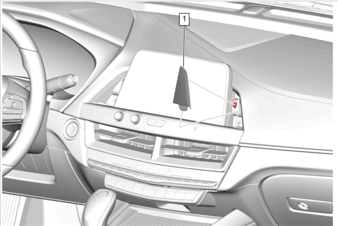
10. Instrument Panel Radio Front Trim Plate (1) » Install
