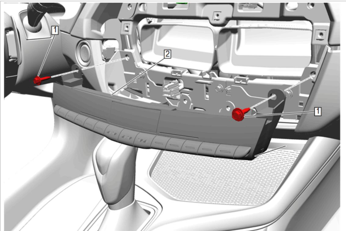
11. Heater and Air Conditioning User Interface Control (2) » Remove
