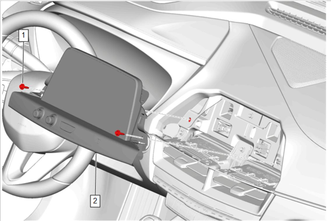
8. Radio Control Bolt (1) » Install and tighten [2x] – Fastener Specifications
