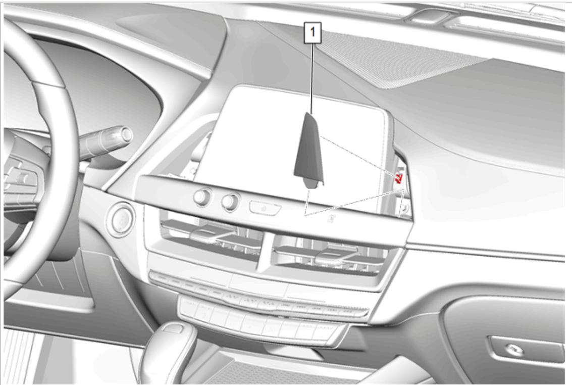
4. Instrument Panel Radio Front Trim Plate (1) » Remove
