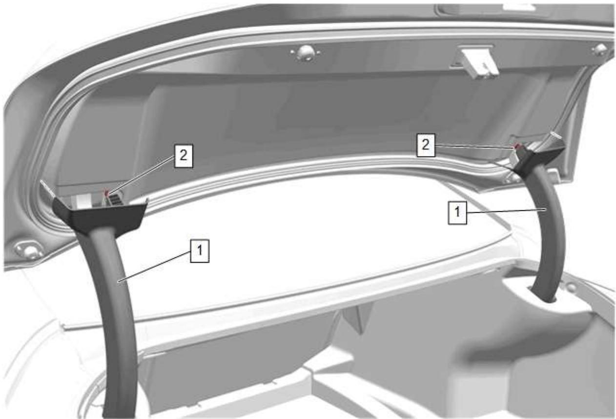
3. Use a small flat-bladed tool at the top of the rear compartment lid hinge cover (1) to release the hinge cover retainer (2) on both sides of the vehicle.
